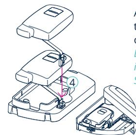
Attach (4.) the cable of the KPC adapter in the slot of the key bed or drawer (depending on variant).
