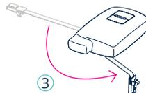
Bend the KPC's cable (3.) around the bottom of the key fob.
