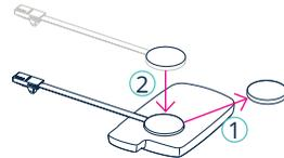
Replace the key fob battery (1.) for proper sized KPC-Adapter (2.).
